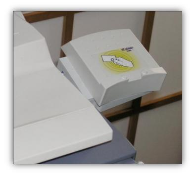
The **Cartadis TCM2 is a**n USB reader of contactless cards for the use of RFID cards, it allows to use the cards already circulating in a firm for a user authentication.
