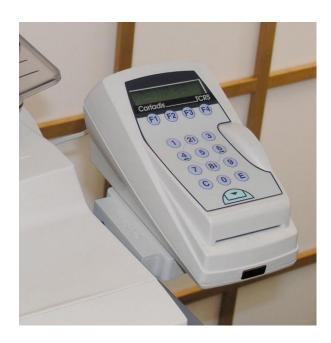
**The magnetic card reader Cartadis TCMIRS** is dedicated to print and copy payments by using a Cartadis magnetic card. This reader is supplied with a networkable interface, **CMI**, for controlling access to printers and MFP. **TCMIRS** is well suited to printing solutions.
