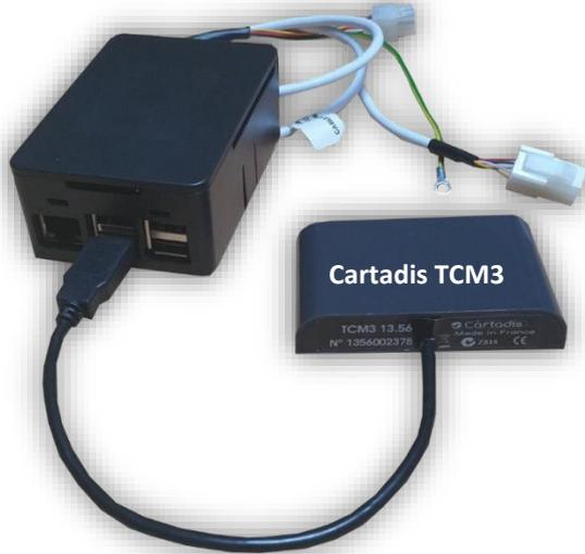
To operate, **cMDB** has to be connected to a card reader, most often a Cartadis reader of contactless cards as shown on the photo (TCM2 or TCM3).
