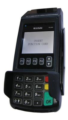
**Cartadis TLC6N** reloads contactless cards or creates wash codes used on the **TL12** terminal to control a gantry. The **TLC6N** equipment is also compatible with the **DJ3** token dispenser, the **TL14** terminal and the **TCM2-CSHP** reader for high pressure and vacuum terminals.
